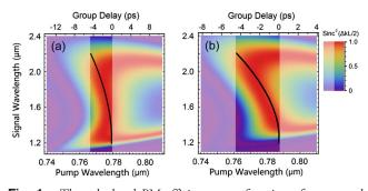
**Fig. 1.** The calculated PM efficiency as a function of pump and signal wavelengths for (a) the collinear configuration (PM angle  $\theta = 10.9^{\circ}$ , noncollinear angle  $\alpha = 0^{\circ}$ ); and (b) the noncollinear configuration (PM angle  $\theta = 10.82^{\circ}$ , noncollinear angle  $\alpha = 0.6^{\circ}$ ). The black line represents the chirped signal pulse with its corresponding wavelengths marked by the left axis and its temporal chirp marked by the top axis.
