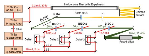
Fig. 3. Schematic setup of the OPCPA system. BS1, 20% reflection beam splitter; BS2, 10% reflection beam splitter; Si BW, silicon window at Brewster's angle.
