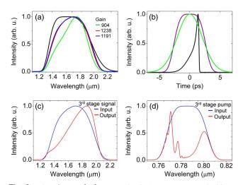
**Fig. 2.** Simulation of a first-stage OPCPA in a 5 mm BIBO: (a) input signal spectrum (black) and output signal spectrum when pumped by 775–785 nm (red), by 760–810 nm (blue), and by 730–830 nm (green); (b) temporal shape of the signal input pulse (black), the 775–785 nm and 760–810 nm pump pulse (purple), and the 730–830 nm pump pulse (green); (c) and (d) simulation of a third-stage OPCPA in a 3 mm BIBO.
