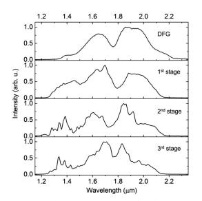
Fig. 4. Spectra taken at successive stages of the laser system.
