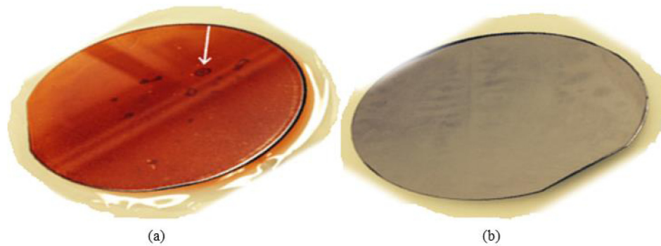
Fig. 6. Voids resulting from poor wafer parallelism when bonding GaP wafers (a); voids are rarely present when bonding GaAs wafers (b).
