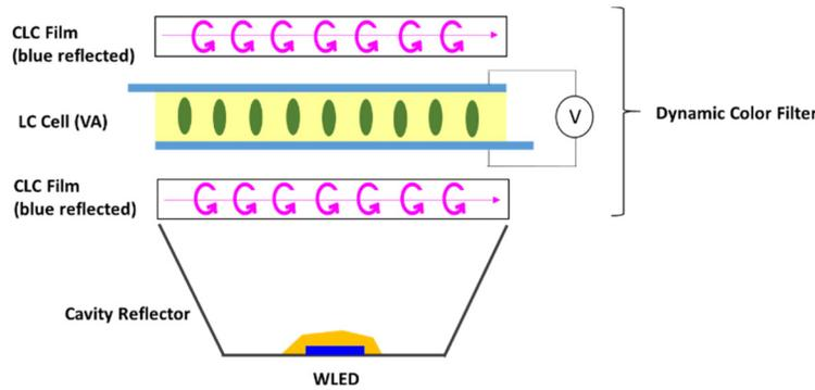
Fig. 1. Device configuration of the proposed CCT tunable WLED using a dynamic color filter.
