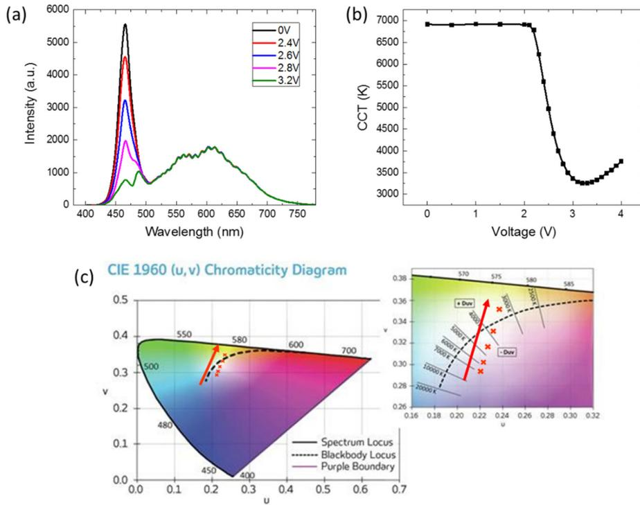
Fig. 4. (a) Measured spectral power distribution of white light with different voltages, (b) relationship between CCT and applied voltage, and (c) CCT in C.I.E. 1960 chromaticity diagram obtained by different applied voltages.
