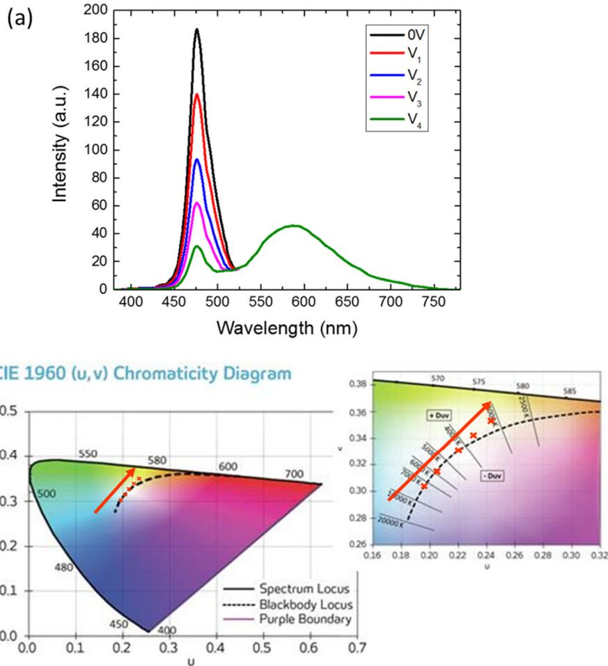
Fig. 6. (a) Simulated spectral power distribution of white light with different voltages, and (b) CCT in C.I.E. 1960 chromaticity diagram with different voltages. In (b), the magnified chart shows how closely the CCT follows the blackbody locus.
