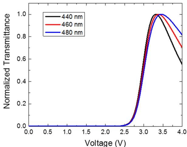
Fig. 7. Voltage-transmittance curves for VA cell at three specified blue LED wavelengths.
