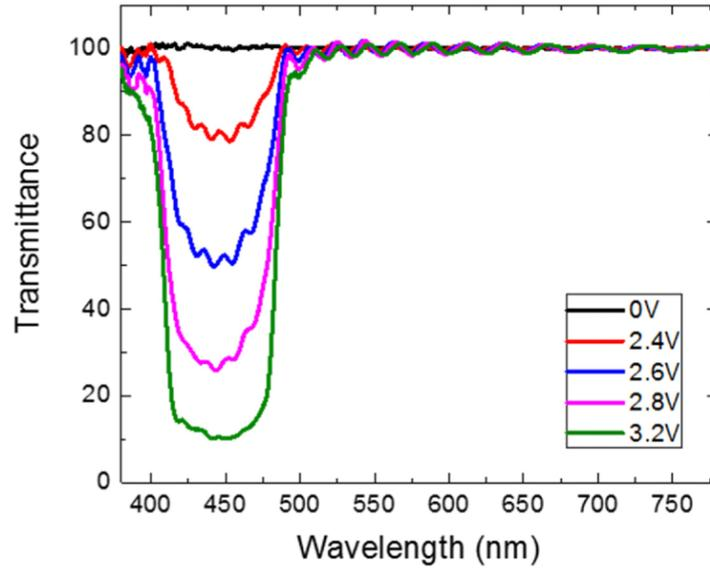
Fig. 3. Measured transmission spectra of the dynamic color filters under different voltages.
