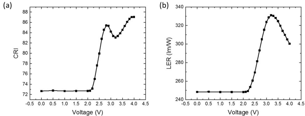
Fig. 5. Measured (a) CRI and (b) LER of the light source with different voltages.
