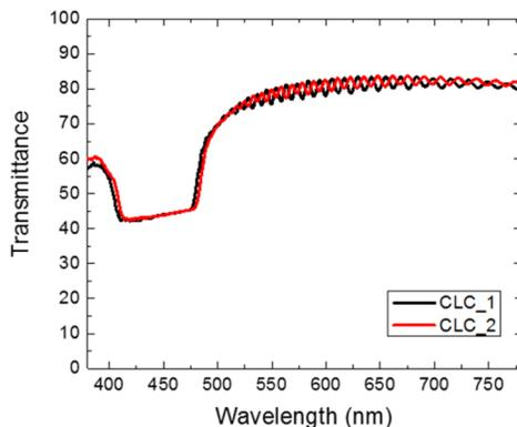
Fig. 2. Measured transmission spectra of two cholesteric liquid crystal films.
