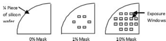
Figure 7. Masks (a quarter size of 100 mm wafer) with varied degree of exposure windows to RIE.
