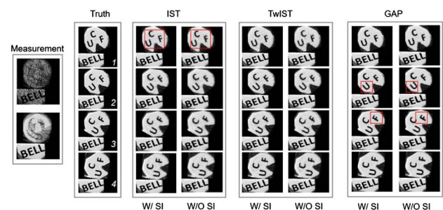
Fig. 4. Measurements and reconstructed video frames with different algorithms for synthesized “BELL-UCF” video with N_T = 4 compared with the ground truth. Notice the quality improvement with SI inside the red rectangles.
