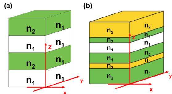
**Figure 5.** The device structure of (a) a reflective polarizer and (b) a functional reflective polarizer.
