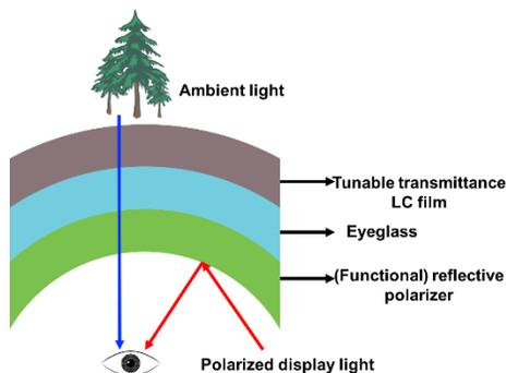
Figure 1. Structure of the proposed AR system
