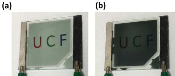
**Figure 4.** The performance of the guest-host LC cell at (a) bright state ( $V=0$ ) and (b) dark state ( $V=8V_{rms}$ ).
