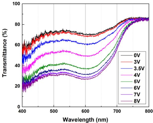
**Figure 3.** Voltage-dependent transmittance of the LC cell.
