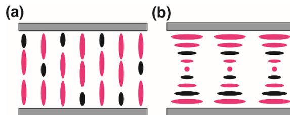
Figure 2. Working principle of the tunable transmittance LC film at (a) bright state and (b) dark state.
