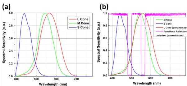
Figure 7. Spectral sensitivity of people with (a) normal vision and (b) protanomaly, the magenta line is the transmittance of the functional reflective polarizer for the transmission state.
