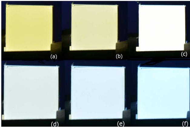
Fig. 4. Experimental results of the output white light with color temperature of: (a) 4909 K, (b) 5507 K, (c) 6493 K, (d) 8016 K, (e) 11,014 K, and (f) 29,715 K.
