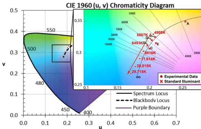
Fig. 5. CIE1960 chromaticity diagram of the tunable CCT by adjusting the proportion of  $W_1$  and  $W_2$  in the mixed white light.
