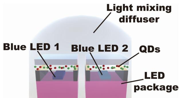
**Fig. 1.** The proposed CCT-tunable QD lighting scheme.
