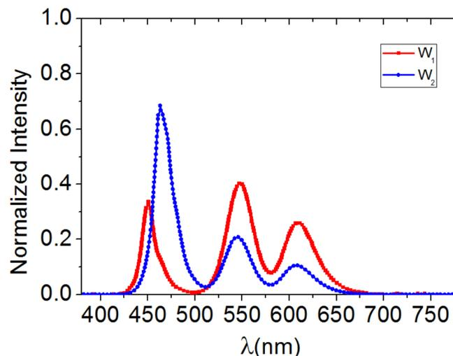
**Fig. 3.** Recorded white light spectra excited by LED B1 ( $W_1$ ) and by LED B2 ( $W_2$ ).
