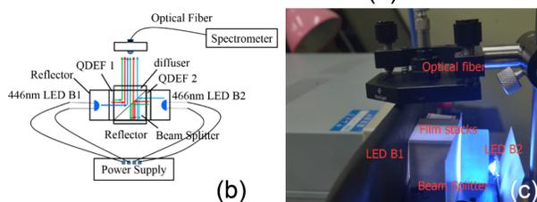
**Fig. 2.** (a) Emission spectrum of R, G QDs and exciting blue LEDs; (b) Schematic drawing of experimental setup and (c) experimental setup.
