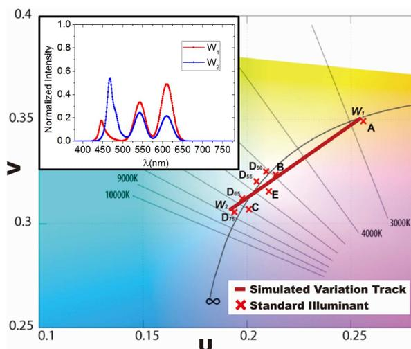
**Fig. 6.** Simulated CCT variation track in CIE 1960 by using red QDs with central wavelength of 626 nm. (Embedded: new  $W_1$  and  $W_2$ )
