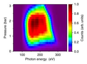
**Fig. 2** Pressure-dependent soft X-ray yield. Soft X-ray continua generated by polarization gating as a function of pressure in the neon gas cell. The spectra were recorded by an electron TOF spectrometer and corrected for the photoionization potential ( $21.6\,\mathrm{eV}$ ) and absorption cross section of the neon detection gas. Photons with energy <100 eV were filtered out using a 100 nm tin filter
