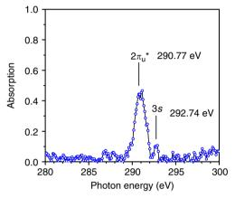
**Fig. 4** Carbon dioxide K-shell photoabsorption spectrum. The two absorption peaks correspond to  $C_{1s} \rightarrow 2\pi_u^*$  and  $C_{1s} \rightarrow Rydberg 3s state^{26}$ . Carbon dioxide gas with 25 torr·mm pressure-length product is used in this measurement
