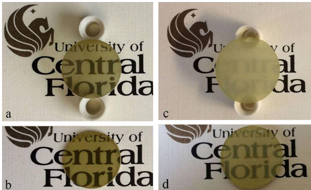
Fig. 6. Photographs of PMN–PT ceramics made from (a and b) combustion-synthesized lead oxide nanopowders; (c and d) and from commercial lead oxide. ( 92 \times 120 \text{ mm}^2 (300 \times 300 DPI)).
