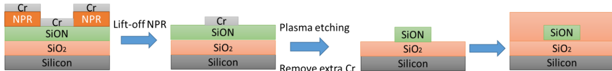
Fig.2 Schematics of the main fabrication processes.
