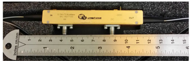
Fig. 1. A fully-packaged commercial LN EO Mach-Zehnder modulator. The total packaged length is \sim 13 cm, and the internal LN chip is \sim 9 cm long. The long length is a consequence of high voltage-length product, and high bending radius; both of these shortcomings of conventional LN waveguides are addressed through the presented thin-film platform.
