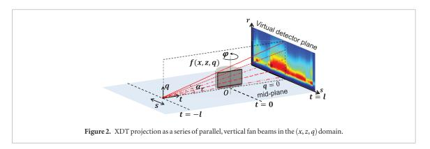
beam. To resolve the complete object function, f(x, z, q), the sample needs to be translated across the beam by the distance s in the (x, z) plane, and rotated around the vertical axis by the angle  $\phi$  similarly to that in a pencil-beam CT. The total number of photons collected by a detector pixel under sample offset s and projection angle  $\phi$  is
