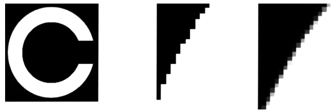
Figure 4. Aliasing and anti-aliasing effect.
