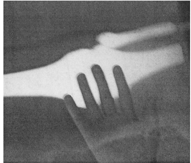
Fig. 3. Natural occlusion of computer-generated object (bone) by real object (hand) in HMPD. Such occlusion is not achievable in conventional see-through displays.
