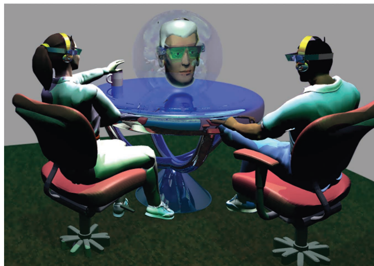
3 Users within the ARC have turned their body toward a real silvered ball painted with optical material and are engaged in an augmented reality experience with a remote user.
