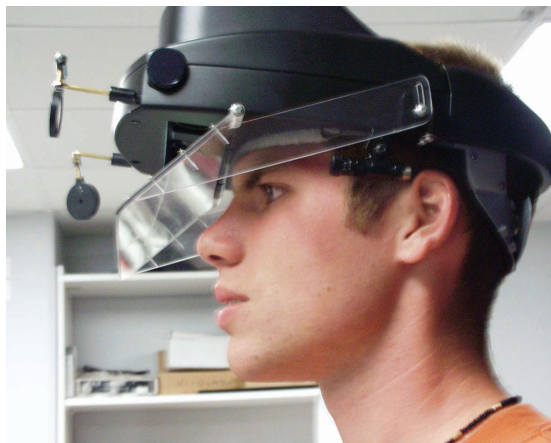
1 Close view of a user wearing a Teleportal HMPD.
