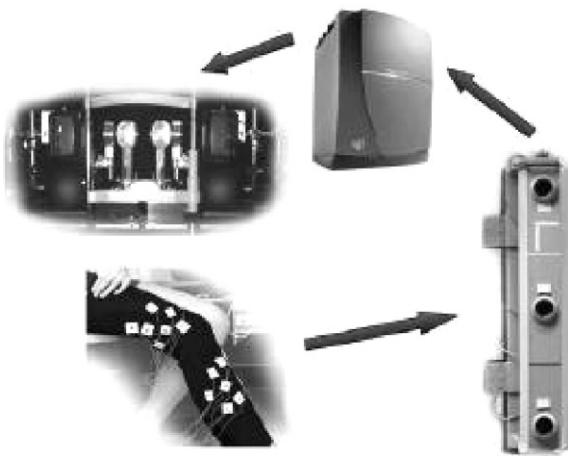
Fig. 4. The VRDA Tool: from markers on a real leg to a see-through head-tracked bench-mounted display.
