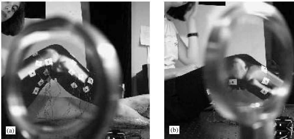
Fig. 6. A flexion (a) and partial extension (b) of the leg of a model patient demonstrating the optical superimposition of knee joint anatomy on a real leg.
