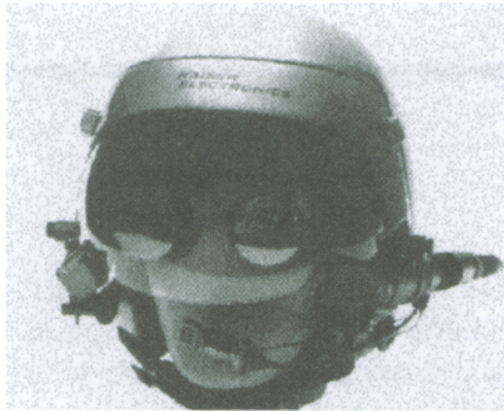
Figure 1. Optical see-through head-mounted display (Photo courtesy of KaiserElectro-Optics).
