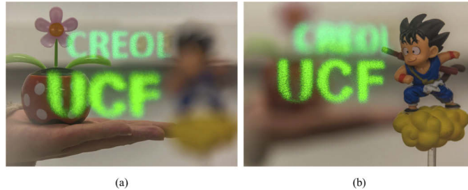
Fig. 4. Photos captured through the near-eye display prototype, where the camera focuses at around (a) 2 m and (b) 1 m in front of the beam splitter.
