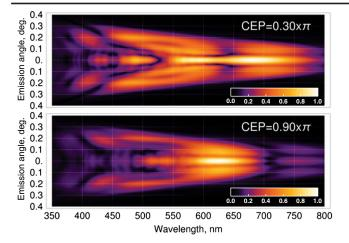
FIG. 2. Numerical results for the  $\theta$ - $\lambda$  spectra, shown on an arbitrary linear scale, for two particular values of the input CEP that correspond to the most dissimilar spectra. The color palette is chosen to highlight the generated spectral features. A movie composed of the  $\theta$ - $\lambda$  spectra for gradually advancing values of the CEP is available in Ref. [27].
