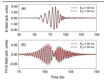
FIG. 5. The simulated complete (a) and third-harmonic (b) output fields, for the input CEP =  $0.30 \times \pi$  and at two different energies of the input pulse, as specified in the legends. 10% energy variation causes only a very slight change of the output waveforms, both in amplitude and phase.
