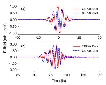
FIG. 3. (a) The simulated *E*-field waveforms for the two values of the CEP that correspond to the two output  $\theta - \lambda$  spectra shown in Fig. 2. (b) Corresponding output *E*-field waveforms of the on-axis emission component. Input pulse energy is 1.40 mJ. The overall CEP of the waveform is rigidly locked on passing through the filamentation zone.
