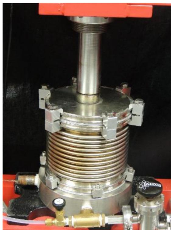
Fig. 2. Vacuum-compatible compressible container used in the sintering experiments. Feedthroughs for a vacuum and gas line along with thermocouple are shown connected to the base. A die press is shown pressing on the vessel which in turn applies pressure on a steel die located inside.
