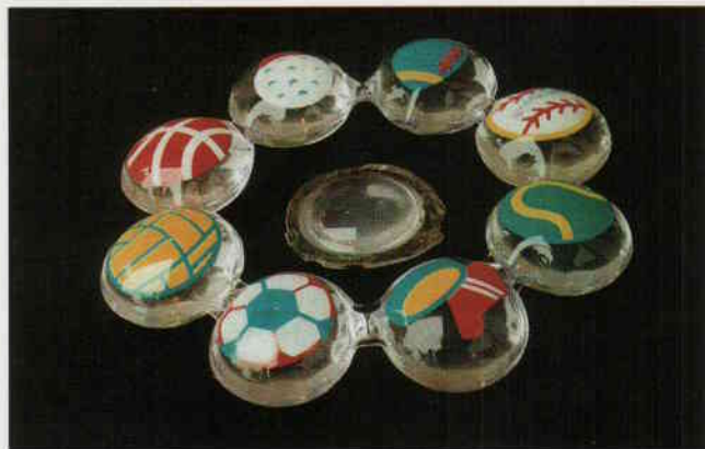
Fig 1a. —Photograph of a water-filled deformable lens in the center of a teething ring. The water-filled deformable lenses were made from transparent teething rings that did not have the imprinted design.
