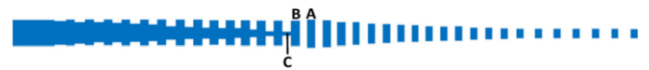
Fig. 17. Schematic of a SOI edge coupler based on SWG [64] (Copyright in 2015, OSA).
