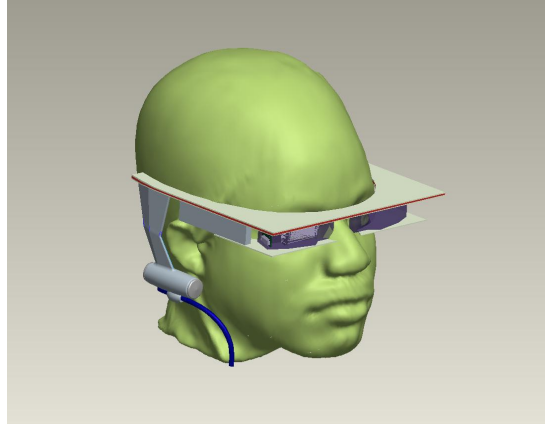
Fig. 5. Opto-mechanical design of a quarter-VGA resolution display
