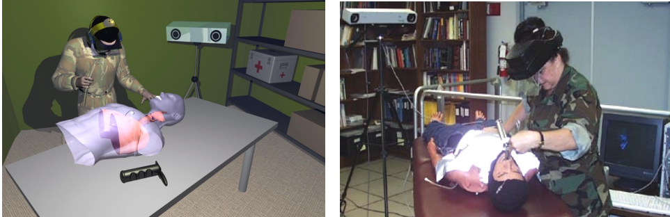
Fig.1 (a) Illustration of the UIH for training paramedics on endotracheal intubation, Graphics by Steve Johnson -ODALab. (b) The system setup, consisting of a HPS dressed with retroreflective material, an optical Polaris tracker, a desktop computer, a HMPD worn by a trainee, and the intubation tools.
