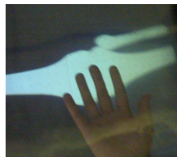
Fig.4 A real object (hand) in front of the virtual object (bone) occludes the virtual object in HMPDs
