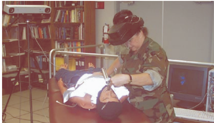
Figure: 3 The system setup, consisting of an optical tracker, desktop computer, HMPD, and curvature measurement device
