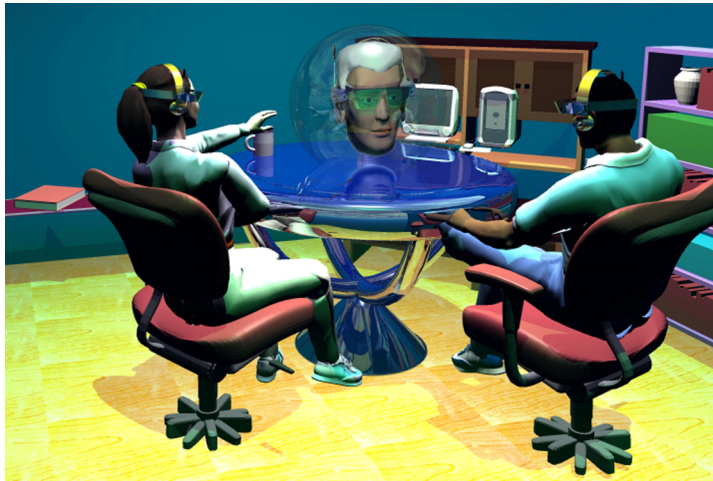
Fig. 2 Illustration of a remote collaborative environment with teleportal capability where a third user's face from a remote site is perceived by each user in the local environment. (Graphics by Stephen Johnson, ODALab-UCF).
