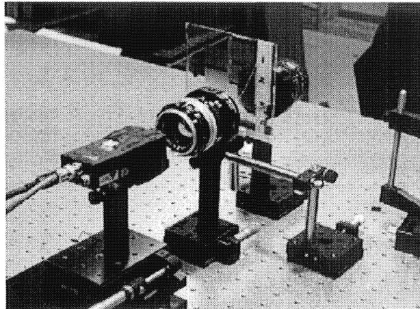
**Figure 2.** The experimental setup used to encode optical phase plates in images.
