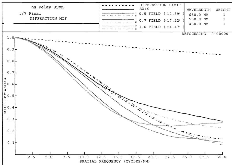
**Figure 3.** MTF Performance of the custom designed relay lens.
