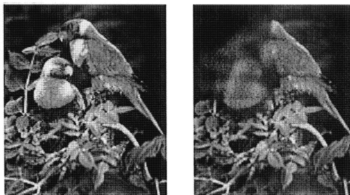
**Figure 7.** Raytrace in ASAP using an optical phase plate covering the upper left  $\frac{1}{4}$  of the object (right) and the original picture (left).
