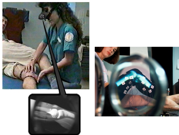
Fig. 1: (a) The VRDA tool allows superimposition of virtual anatomy on a model patient. The inset photograph contains a rendered frame of the knee-joint bone structures animated based on a kinematic model of motion. (b) An actual view from the VRDA Tool from the viewpoint of the user.
