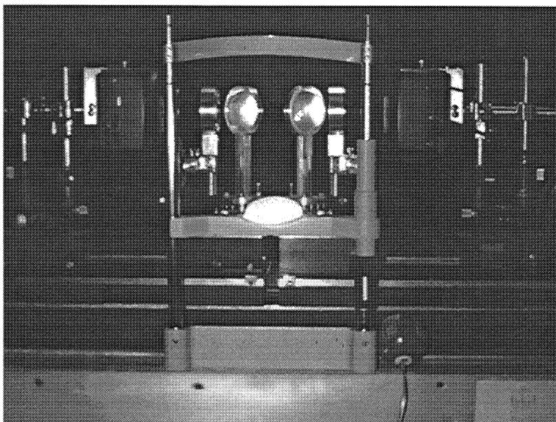
**Figure 1.** *Experimental setup. Shown is a chin rest for the human subject, the optical viewer, two LCD displays, and a two-button input device in the form of a ball for easy handling.*
