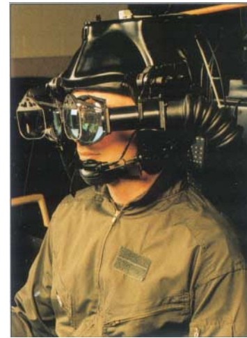
Fig. 3 Fiber optics HMD. Courtesy of CAE electronics. (View this art in color at www.dekker.com .)
