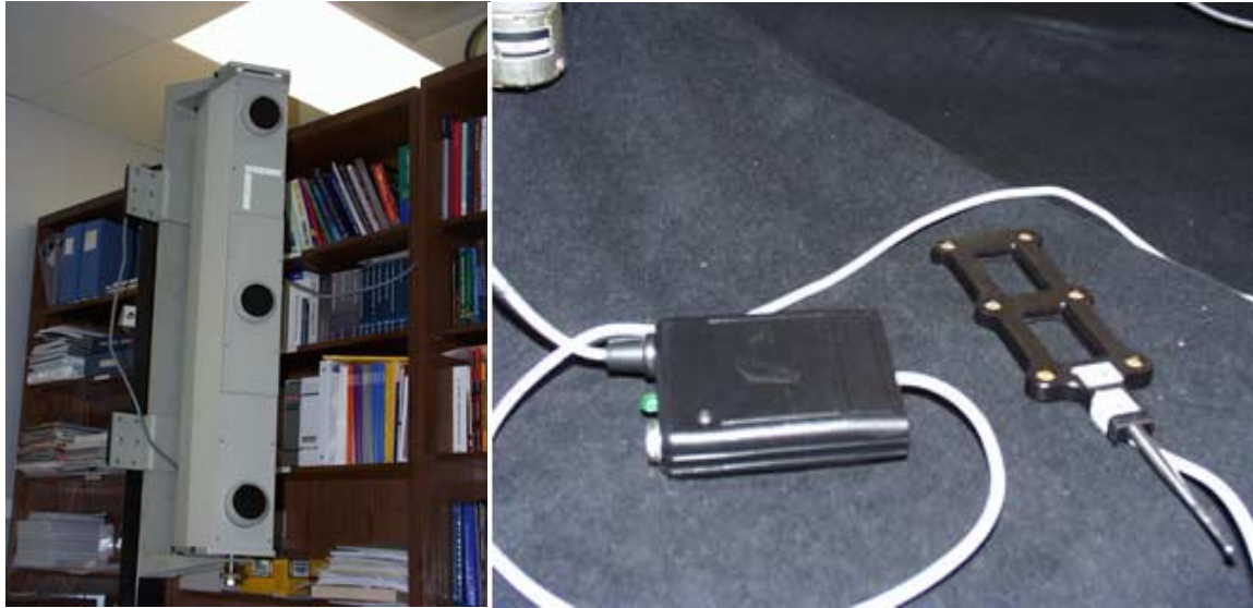
Figure 21: The Optotrak 3020 from Northern Digital (left frame) mounted on a stand with its three cameras. A rigid body or tracking probe (right frame) with 6 markers and the control device to fire the LEDs.
