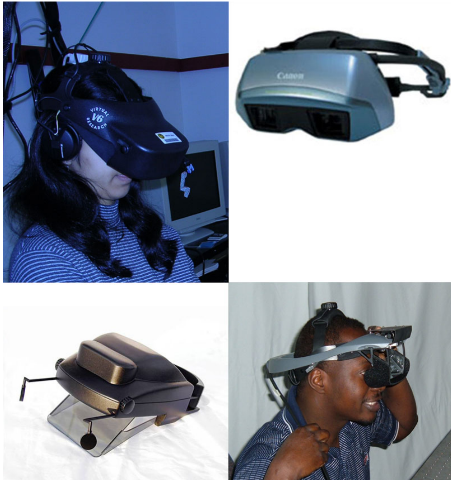
Figure 22 The upper left panel shows the VR6. The upper right panel shows the Canon Coastar. The bottom two panels show the ODALab prototype displays, on the left the HMPD-1 and on the right the HMPD-2, respectively.
