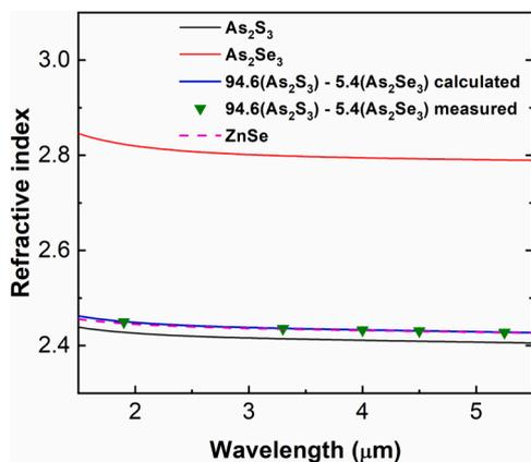
Fig. 1. Refractive indices of  $\text{As}_2\text{S}_3$ ,  $\text{As}_2\text{Se}_3$ , ZnSe, and that of a ternary As-S-Se mixture in the mid-IR spectral region.
