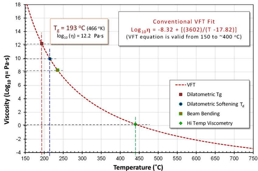
Fig. 3. Viscosity curves in function of temperature of the chalcogenide base glass using a VFT fit.
