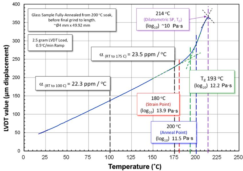
Fig. 2. Thermomechanical dilatometry curve of the base chalcogenide glass as a function of temperature.
