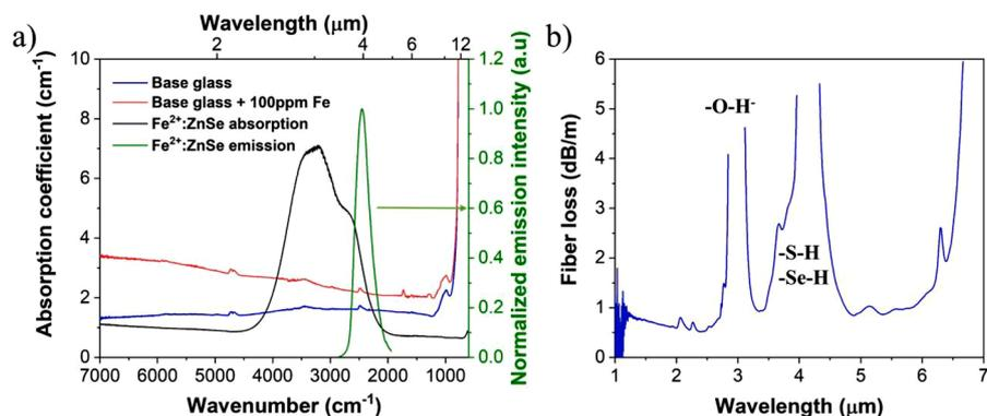
Fig. 4. a) Absorption coefficient of BG with and without iron doping with the absorption and the mid-IR emission bands for  $\text{Fe}^{2+}$  in ZnSe crystals at 77K; b) IR fiber loss of BG optical fiber
