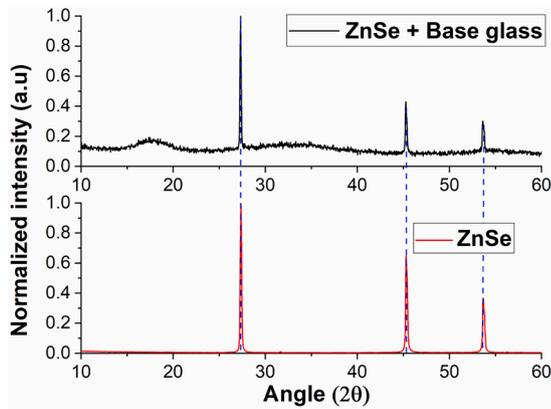
Fig. 6. XRD data of (top) ZnSe mixed with BG powders after heat treatment at 360C for 30 min and (bottom) reference spectra for ZnSe powders.
