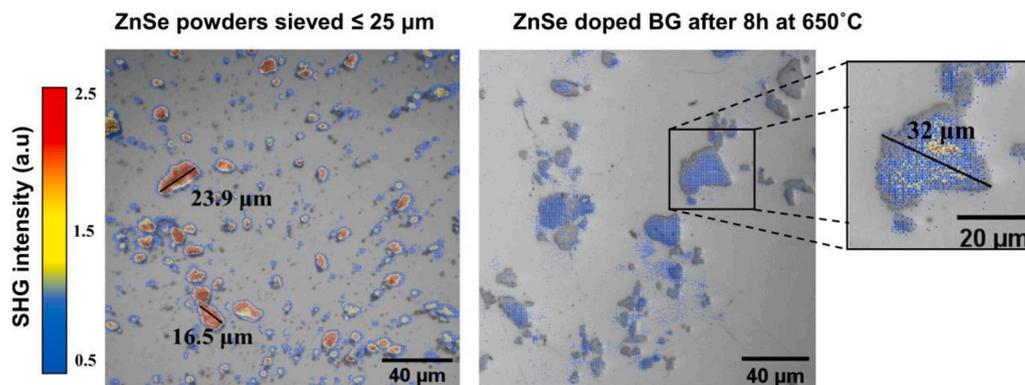
Fig. 7. Combined optical microscopy and SHG images (left) of post-sieved ZnSe particles passing through a 25 $\mu\text{m}$  sieve, on a microscope slide and (right) SHG map (dots) representative of ZnS/ZnSe particles in a ZnSe doped As-S-Se base glass after remelt for 8 h at 650C of the mixture. The scale bar and drawn lines illustrate the length scale of the features shown. The colors of the regions are representative of the SHG intensity.
