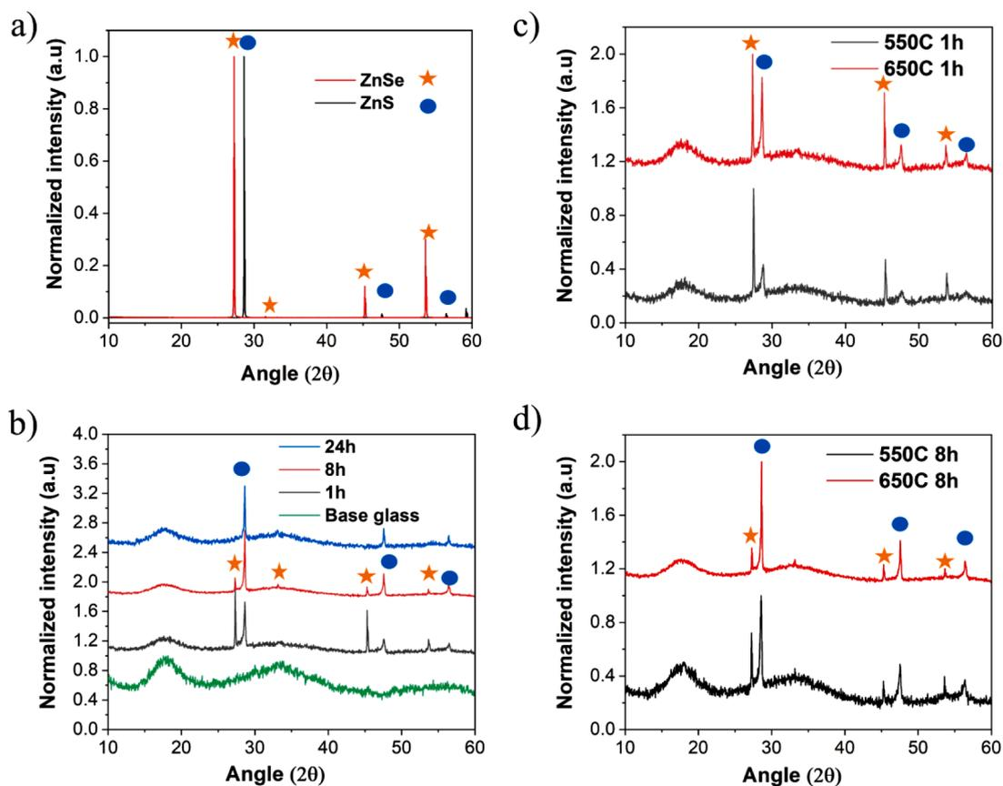
Fig. 5. XRD data of a) ZnSe and ZnS crystals, b) ZnSe-doped BG melted at 650C for 1, 8 and 24 h, c) ZnSe-doped BG melted at 550 and 650C for 1 h and d) ZnSe-doped base glasses BG melted at 550 and 650C for 8 h. Diffractograms on graphs b), c) and d) were vertically shifted for clarity.
