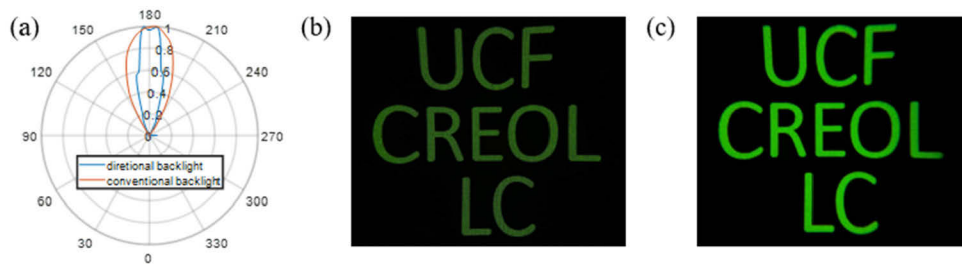
Fig. 5. (a) Normalized angular distribution of conventional BL and directional BL. Imaging results of Fresnel system with (b) conventional BL, and (c) directional BL. The horizontal FOV of the images in (b) & (c) is around \pm 15^\circ .
