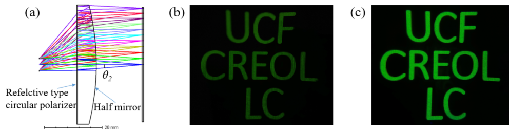
Fig. 9. (a) Zemax profile of the “Pancake” lens. Imaging results of “Pancake” system with a (b) conventional BL and (c) directional BL. The horizontal FOV of the images in (b) and (c) is \pm 23^\circ .
