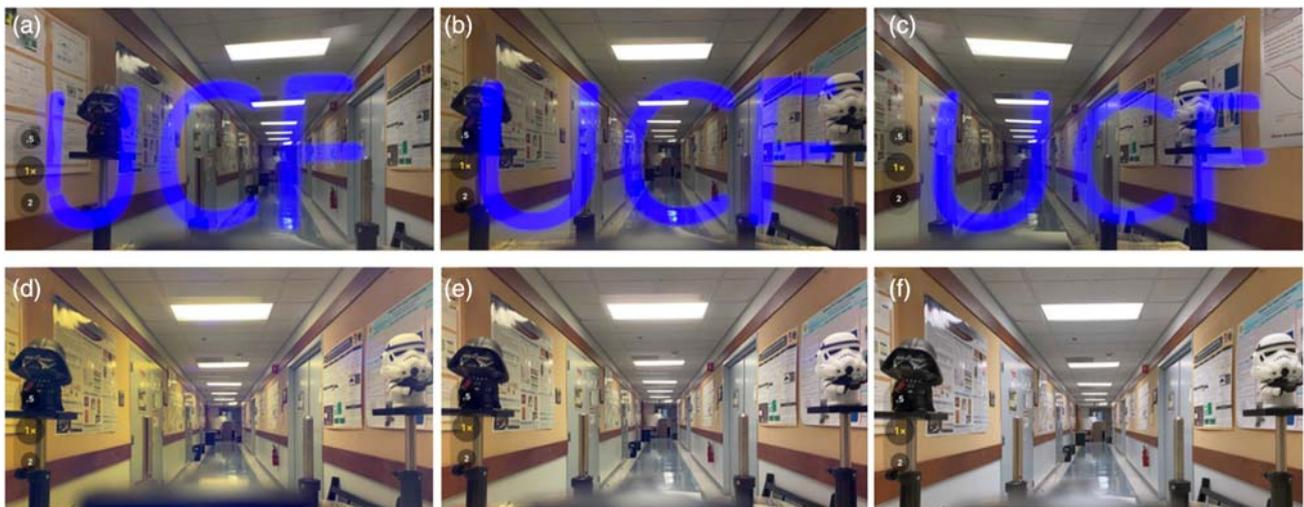
**Figure 11.** a–c) Photos of the imaging results with a low diffraction efficiency optical combiner. Photos of real environment background with a: d) high diffraction efficiency combiner, e) low diffraction efficiency combiner, and f) no optical combiner.
