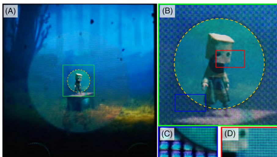
FIGURE 7 Experimental photographs of the proposed multi-resolution display with 4.4\times resolution enhancement: (A) whole displayed image; (B) the magnified green square region in (A); (C) the magnified blue rectangle region in (B); and (D) the magnified red rectangle region in (B)
