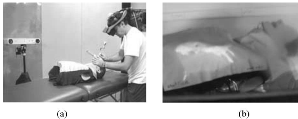
Fig. 5. (a) System components. (b) User's view (augmented) captured with a camera placed behind one eye in the HMD.
