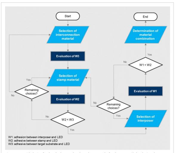
**Figure 18.** Material selection flowchart for the stamp-based transfer process. The flowchart starts with the selection of an interconnection material. Reproduced from [169], with permission from Springer Nature.
