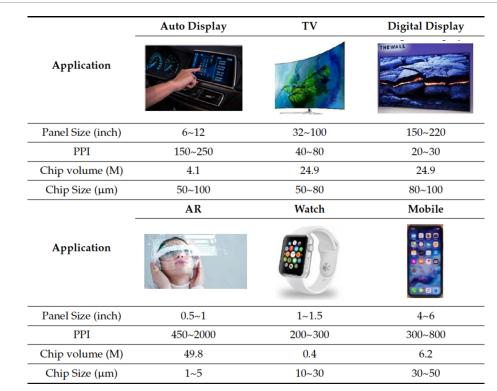
Figure 14. Requirements for micro-LEDs in typical applications [125]. Some related specifications can be found in other separate sources, for example, the TV and signage [132], the AR goggles [109], and the smartwatch [133]. Reproduced from [125]. CC BY 4.0.
