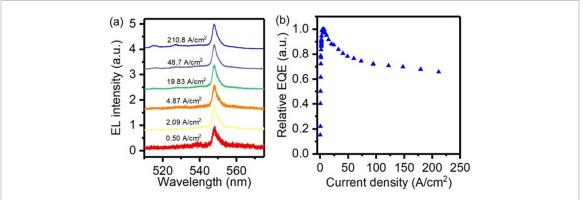
**Figure 6.** (a) Electroluminescence spectra of an InGaN/GaN photonic nanocrystal micro-LED measured under varying injection current at room temperature. (b) Variation of the relative external quantum efficiency (EQE) vs. injection current density. Reprinted from [51], with the permission of AIP Publishing. © [2022] IEEE. Reprinted, with permission, from [43].
