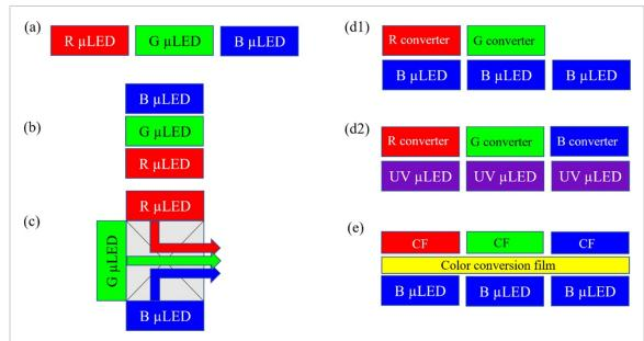
**Figure 12.** Schematics of (a) side-by-side RGB  $\mu$ LEDs. (b) Stacked RGB  $\mu$ LEDs. (c) Three-panel system. (d1) Patterned color converters with blue  $\mu$ LED array. (d2) Patterned color converters with UV  $\mu$ LED array. (e) White light with color filters.
