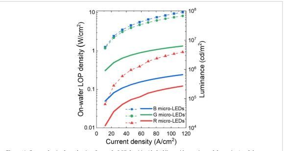
**Figure 10.** Current density dependencies of on-wafer LOP densities (dashed lines with experimental data points) and the luminance (solid lines) for RGB micro-LED arrays.
