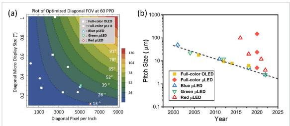
**Figure 23.** (a) Theoretical contour plot of diagonal FOV at 60 pixel per degree (PPD) versus display size and PPI. (b) Pitch size of the full-colored OLED, full-colored micro-LED, blue light micro-LED, green light micro-LED and red-light micro-LED microdisplays.
