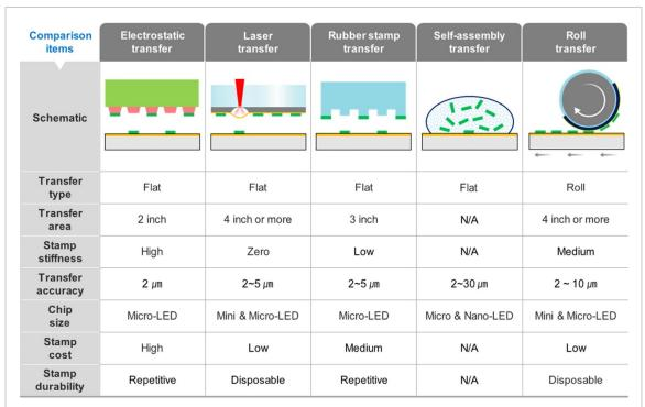
**Figure 17.** Available transfer technologies and their characteristics. The suitable transfer technology depends on target applications' technical specifications. Reproduced from [169], with permission from Springer Nature.
