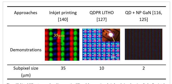
**Figure 15.** List of different approaches of incorporating QDs and the respective subpixel resolutions for micro display. Reprinted with permission from [140]. Copyright (2020) American Chemical Society. Reproduced from [127]. CC BY 4.0. Figure source of QD+NP GaN: Saphlux Inc.
