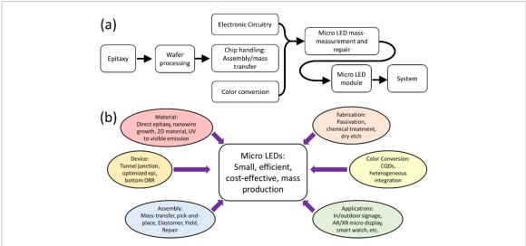
**Figure 2.** (a) A simplified supply chain model for a micro-LED system and the scope of this roadmap. (Source: Industrial Technology Research Institute, Taiwan). (b) The conceptual visualization of what a good micro-LED technology should be. Most of the topics are discussed in this study.
