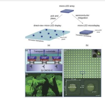
**Figure 11.** Schematics of the pick-and-place approach (top) and the integration of  $\mu$ LED arrays with arrays of transistors (bottom) [90, 91]. [90] John Wiley & Sons. © 2016 Society for Information Display. Reprinted from [91], with the permission of AIP Publishing.
