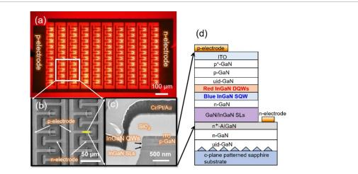
**Figure 9.** Top-down view of InGaN-based red micro-LEDs (17 x 17  $\mu$ m<sup>2</sup>) with (a) and without (b) current injection. (c) Cross-sectional transmission electron microscopy (TEM) image of a single micro-LED device. (d) The InGaN-based red LED structure. Reproduced from [77]. CC BY 4.0.
