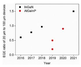
**Figure 3.** The progress in improving the peak EQE of  $20 \times 20 \,\mu\text{m}^2$  InGaN and AlGaInP micro-LEDs at UCSB. The EQE ratio is relative to the corresponding  $100 \times 100 \,\mu\text{m}^2$  devices with indium tin oxide (ITO) contact.
