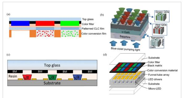
Figure 13. (a) Patterned CLC film on top of color conversion materials. Reproduced from [115]. CC BY 4.0. (b) Nanoporous GaN embedded with QDs. u-GaN refers to unintentionally doped GaN. Reprinted with permission from [116]. Copyright (2020) American Chemical Society. (c) Top black matrix for mitigating color shift. Reprinted with permission from [113] © The Optical Society. (d) Funnel-tube array for reducing color crosstalk. Reproduced from [119]. CC BY 4.0.
