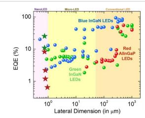
Figure 4. Variations of peak EQE of some previously reported III–V visible LEDs with different lateral sizes. Our results are shown as stars, with the color of the star corresponding to the device emission color. © [2022] IEEE. Reprinted, with permission, from [43].
