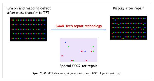
backplane, which can save time comparing to three times bonding process directly onto backplane. The lower process temperature can improve alignment accuracy comparing to heating and cooling for three cycles of directly transfer. In figure 20, our steps to perform this assembly/repair procedure can be illustrated based on our unique chip-on-carrier technique.
