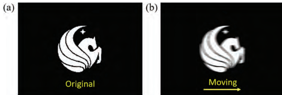
Figure 2. Illustration of motion blur. (a) Original profile of the displayed object. (b) Perceived blurry profile when the object is moving with a high speed in display. Reproduced from Ref. [38], with the permission of the author.
