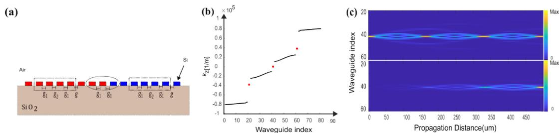
Fig. 1. (a) Silicon photonics superlattice; (b) Propagation-constant spectrum; (c) Propagation simulation of the pump (top) and photon pairs (bottom).
