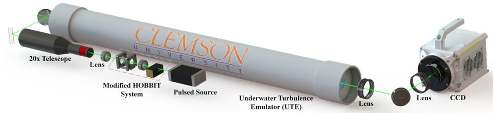
**Fig. 3.** The modified HOBBIT system generates beams that are propagated through a turbulent underwater environment within the non-diffracting region before being captured with a CCD.
