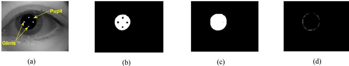
Figure 2: The steps involved in finding the center of the pupil (a) acquire the native eye image (b) threshold the image (c) perform a closing operation to remove holes (d) fit an ellipse to estimate the center and shape of the pupil
