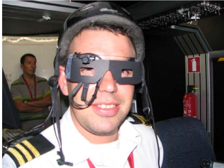
Figure 7: Pilot Wearing Head and Eye Tracking System; With Mask
