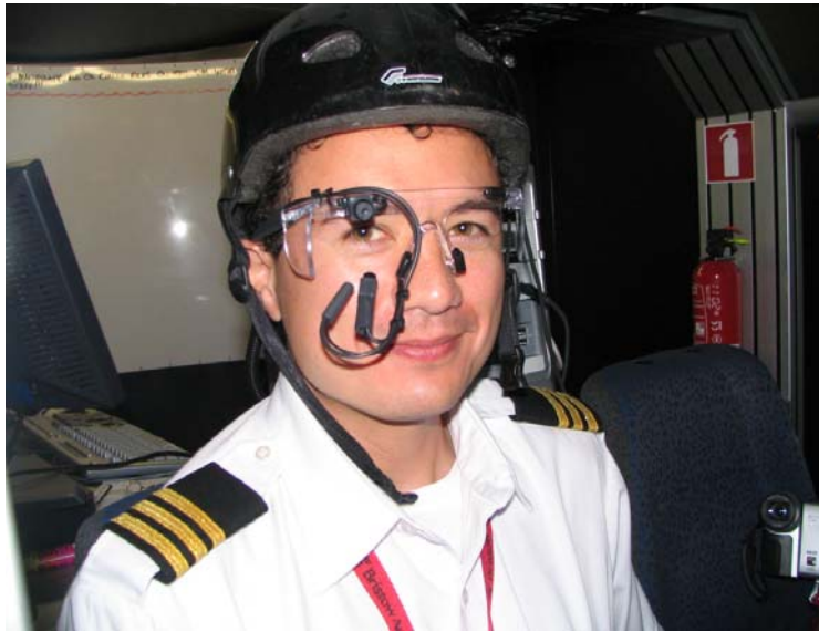
Figure 6: Pilot Wearing Head and Eye Tracking System; No Mask
