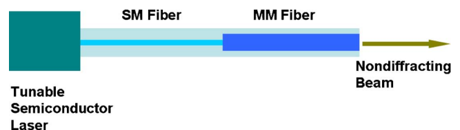
FIG. 1. (Color online) Design of a fiber device generating nondiffracting beams (the figure is not to scale).
