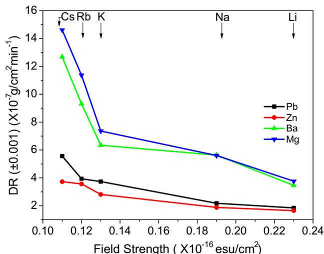
**Fig. 4.** Dissolution rate of  $R_2O$ – $MO$ – $TeO_2$  glasses in deionized boiling water.
