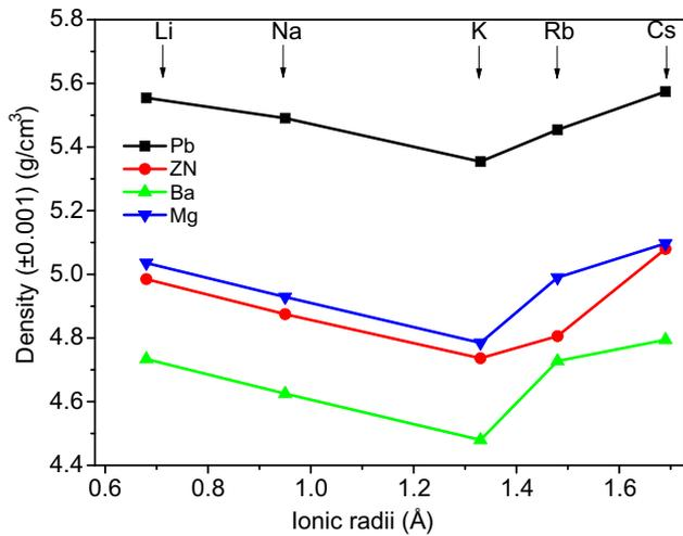
Fig. 7. Density of tellurite glasses introducing several modifiers.
