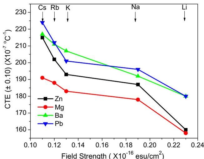
Fig. 2. Coefficient of thermal expansion of tellurite glasses composition.
