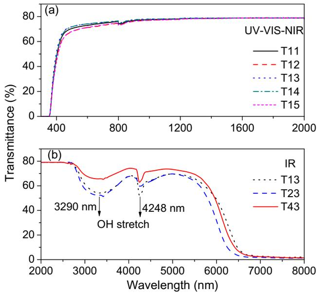
Fig. 5. Transmission spectra in a range of (a) 300–2500 nm and (b) 2000–8000 nm.
