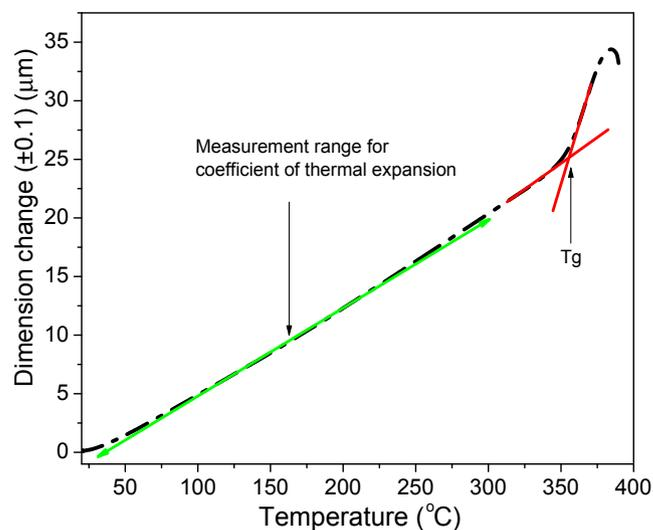
Fig. 1. Thermal expansion and glass transition temperature curve.
