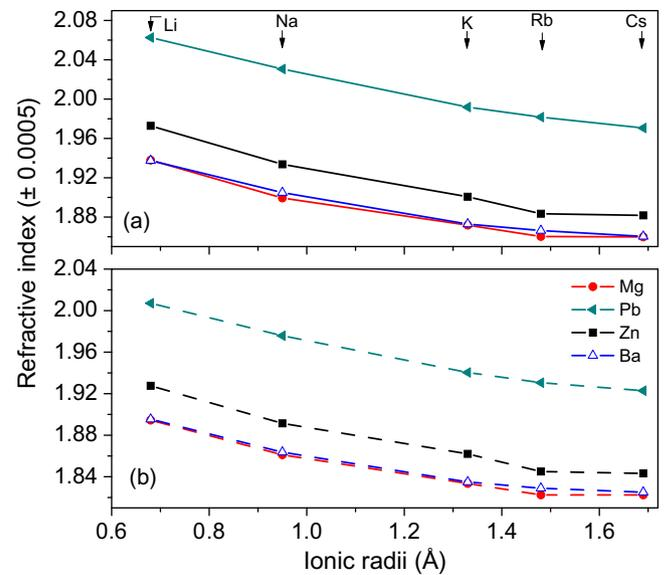
Fig. 6. Refractive index as a function of ionic radii for  $\text{R}_2\text{O-MO-TeO}_2$  glasses at (a) 632.8 nm and (b) 1550 nm.
