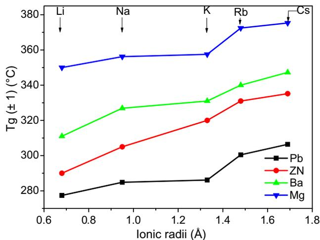
**Fig. 3.** Glass transition temperature ( $T_g$ ) as a function of ionic radii.
