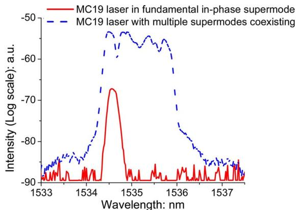
Fig. 4. (Color online) Spectra of MC19 lasers with dual spliced passive fibers (solid curve) and with no modal controlling elements (dashed curve).
