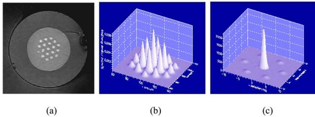
Fig. 2. (Color online) (a) Microscopic image of an active 19-core fiber and calculated (b) near-field and (c) far-field intensity distributions of the fundamental in-phase supermode.
