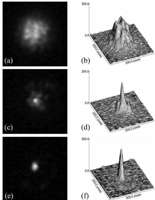
Fig. 3. Far-field intensity distributions of MC19 laser emissions: (a), (b) bare MC19; (c), (d) one end spliced with passive fiber; (e), (f) both ends spliced with passive fibers. (b), (d), and (f) are three-dimensional views of (a), (c), and (e), respectively. All photos are taken at an output level of  $\sim 200$  mW.
