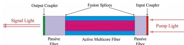
Fig. 1. (Color online) Illustration of the proposed fiber laser device: both ends of a MCF are spliced to passive fibers that are coated with dielectric mirrors (length not to scale).
