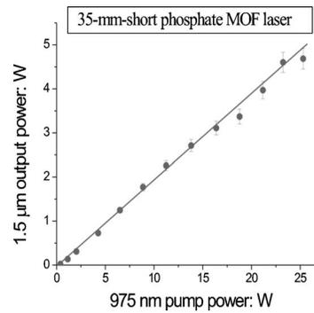
FIG. 3. Signal vs pump plot of a 35-mm-short MOF laser. Dots: experimental data; solid line: linear fit.
