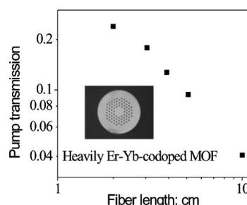
FIG. 1. Pump absorption of the heavily doped cladding-pumped MOF in log-log scale. Inset: photo of the large-mode-area active MOF.
