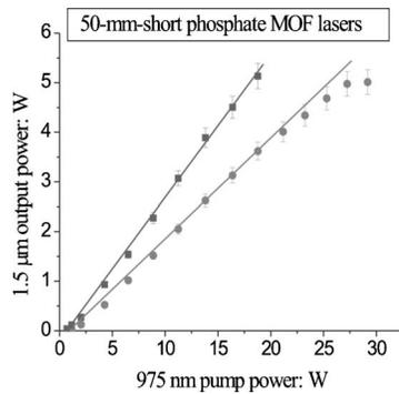
FIG. 2. Performances of two 50-mm-short MOF lasers. Squares: with external OC; dots: without OC; and solid lines: linear fits.
