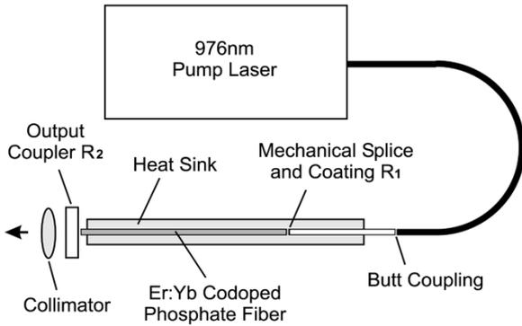
Fig. 2. Experimental setup of the short-length Er–Yb codoped phosphate fiber lasers.
